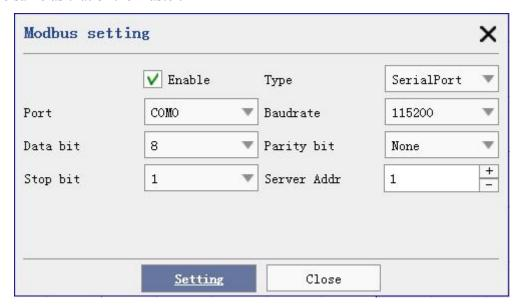
**Serial port mode:** Serial port mode needs to set the connection information of the serial port. The service address needs to be the same as that of the master.
